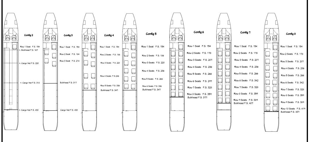
Utilize these drawings to assist in the proper reconfiguration of the aircraft
